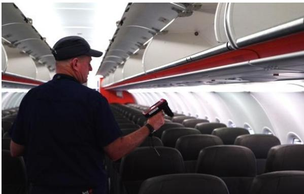
*John Gardner, Jetstar Engineer performing an RFID-enabled cabin scan.*
